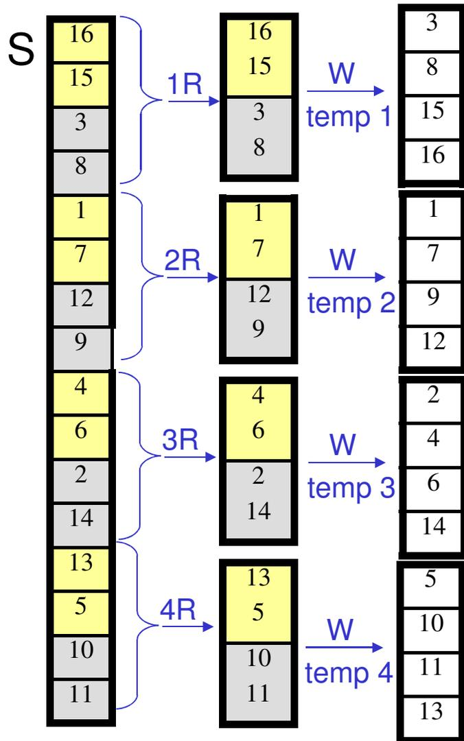
$$\begin{aligned} \text{Custo Total} &= 2 * b_S + \\ &\quad 2 * b_S * \log n_{buf} (b_S / n_{buf}) \\ &= 2 * b_S (\log n_{buf} (b_S / n_{buf}) + 1) \end{aligned}$$
