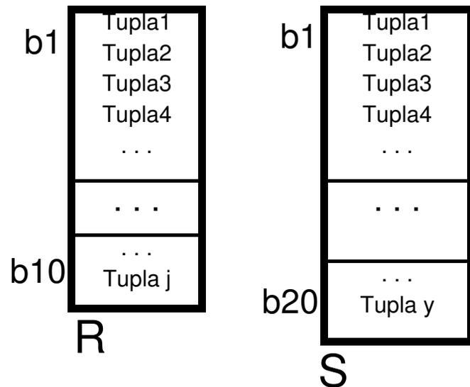
$$\begin{aligned} \text{custo} &= \text{MIN} (10+10*20, \\ &\quad 20+20*10) \\ &= 210 \text{ acessos} \end{aligned}$$
