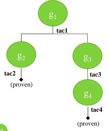
If all leaves are 'closed' (proven) we build the root-theorem by applying the proof functions in the bottom-up way.
