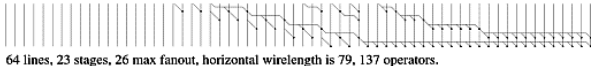
Figure 11: A parallel prefix circuit adapted to a typical delay profile on the output of a reduction tree.
